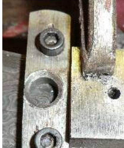
Start with two pieces of steel (here  $\frac{3}{4}$ " x  $\frac{3}{8}$ " x 2.0"). They just have to be thick enough not to bend easily (small angle iron would do), wide enough to drill and tap the bolt holes, and long enough to span the actual blade height plus room for the bolts. The bolts here are 8x32 socket cap screws. I used them because I have a box of a 100. I would not do lighter and anything over  $\frac{1}{4}$  is way overkill.
